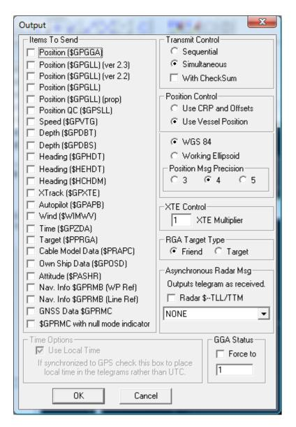
The following items are configurable within this dialog box. These items must be configured for proper data output on the assigned port. You should note that the NMEA OUTPUT device could be added to the WinFrog Computer multiple times, for outputs on various ports.
